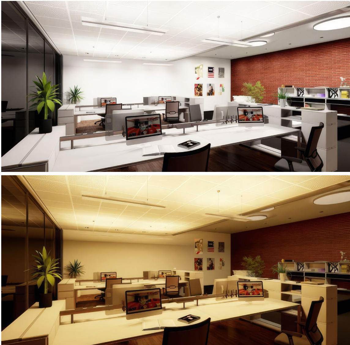
Fig. 5. Extreme lighting scenes: top, a lighting simulation for a circadian activation phase in an office environment; bottom, the lighting programmed for a pre-rest phase or minimum circadian interference.
